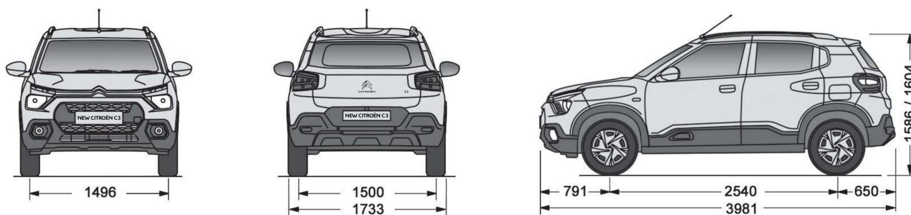
All measurements are in millimetres.
